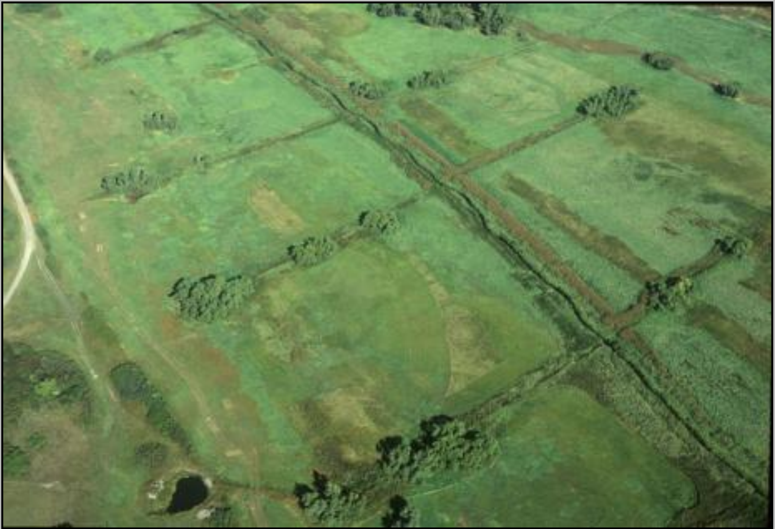
Surface Drainage Ditches in Sandhills wet meadow
